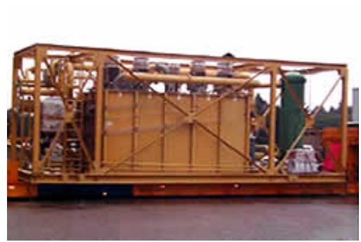
Cooling - heating - filter systems for a steam turbine
