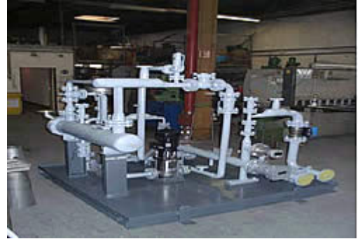
Cooling - heating - filter systems for a centrifugal or piston engine
