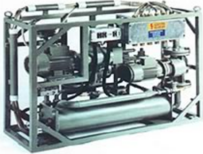
Combined Preheating and Pre-lubricating
